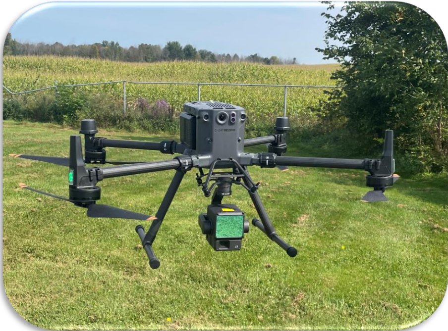
SNC's new DJI Matrice 350 RTK drone with LiDAR camera payload
