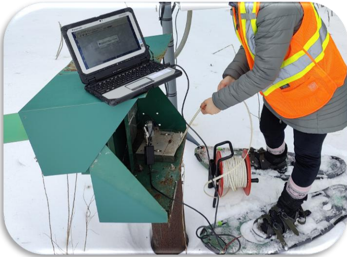
Manual water level measurement, South Dundas
